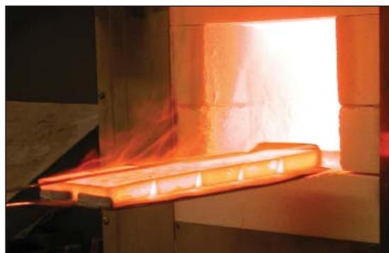
Fig. 2. The precious metal samples are withdrawn from the furnace after the cupellation process has been fully completed
