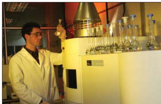
*Fig. 3. Sample preparation for ICP-OES. The chemist is checking for the presence of undissolved sample in the volumetric flask, before subjecting the solution to instrumental analysis*
