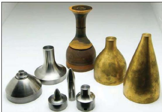
Fig. 2. Formers for spinning parts of the palladium jug, in brass and steel
