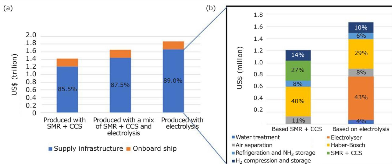
Fig. 1. (a) Aggregate investment for ammonia production *via* different routes; (b) capital cost breakdown for green ammonia production to decarbonise shipping by 2050. Redrawn using data in (3)
