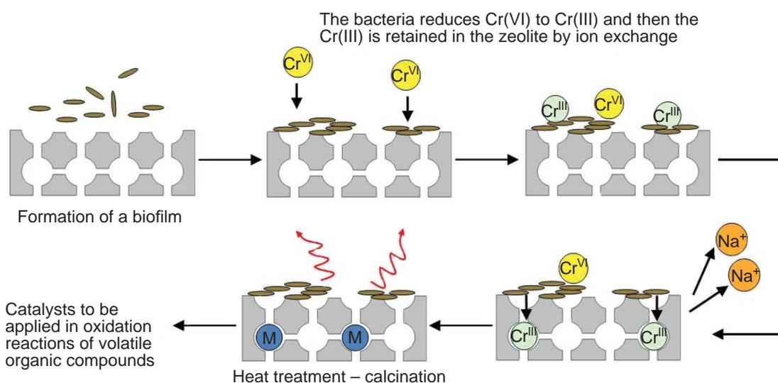
Fig. 1. New method of chromium removal from wastewater and catalytic reutilisation in volatile organic compounds oxidation (Reproduced by permission of Royal Society of Chemistry)
