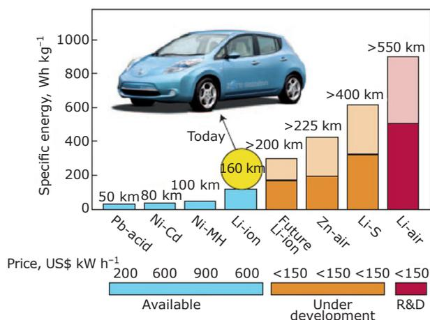
Fig. 1. Practical specific energies for some rechargeable batteries, along with estimated driving distances and pack prices (Reprinted by permission from Macmillan Publishers Ltd: *Nature Materials* (4), copyright (2012))
