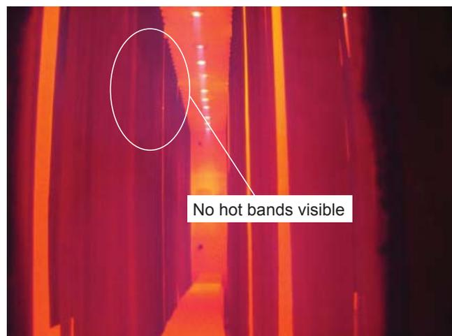
Fig. 6. Tube appearance after plant shutdown and steaming showing conditions returning to normal
