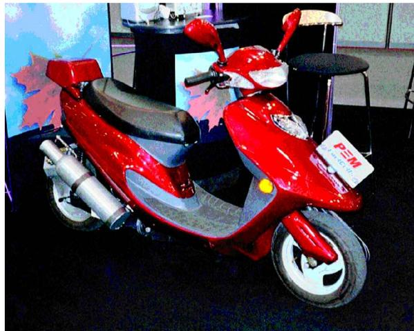
A motor scooter displayed on the PEM Technologies Inc. stand. This company is focusing in particular on small to medium size fuel cell power systems with an electric output of less than 10 kW. The fuel cells are aimed at use in portable power systems, light/personal and non-road industrial electric vehicles
