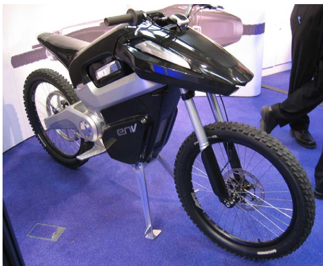
Fig. 1 This ENV motorbike, demonstrated by Intelligent Energy, features a 1 kW PEM-type power pack fuelled by compressed hydrogen. The hybrid design, when used in combination with lead acid batteries, gives a top speed of 80 kmph and a range of over 160 km. The power pack is easily removed for independent use
