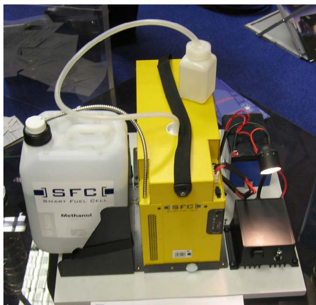
Fig. 3 A direct methanol fuel cell produced by Smart Fuel Cell. This was operated at the exhibition alongside the Symposium. Its output is 50 W at 4 A; methanol consumption is 1.3 \text{ l kWh}^{-1} ; and its overall weight is 8 kg
