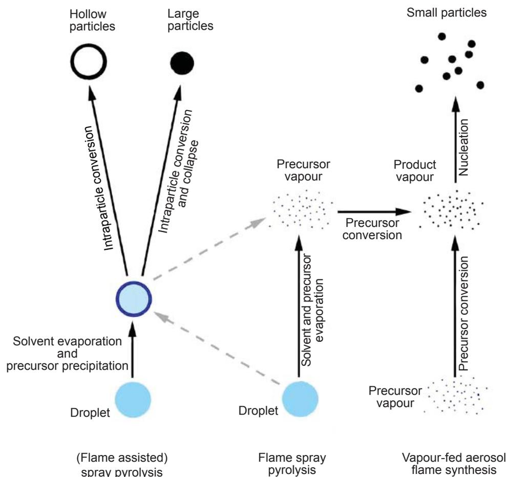
Fig. 6. Mechanism of formation of particles during spray pyrolysis processes (22) (Copyright © 2006 Koninklijke Brill)
