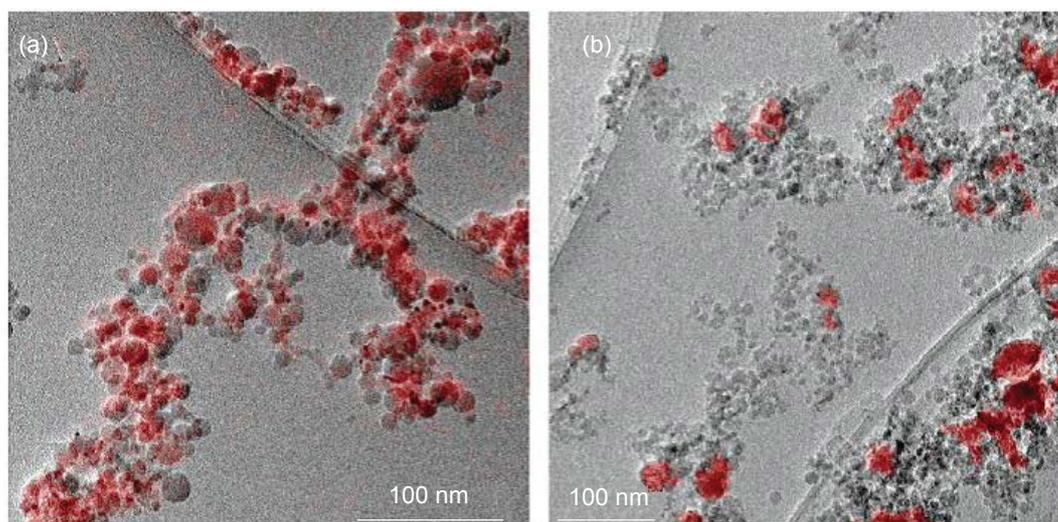
Fig. 9. Transmission electron microscopy (TEM) pictures of Pt/Ba/Al<sub>2</sub>O<sub>3</sub> made with: (a) one nozzle; (b) two nozzles. The red areas indicate the presence of Ba (Reprinted with permission from (75). Copyright (2006) American Chemical Society)
