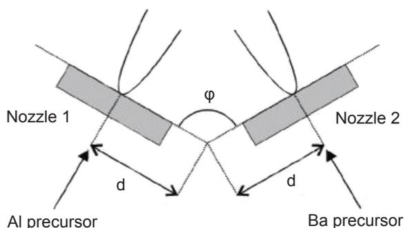
Fig. 8. Scheme of the geometric arrangement of a double FSP set up (Reprinted with permission from (75). Copyright (2006) American Chemical Society)
