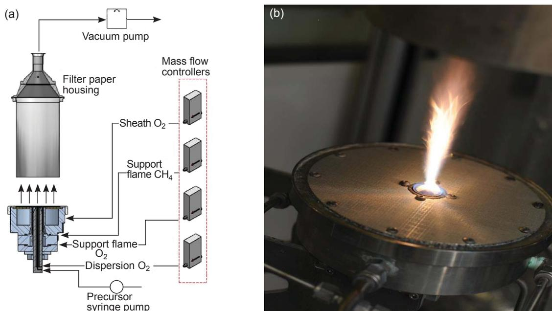
Fig. 1. (a) Schematic of the experimental flame spray pyrolysis setup; (b) picture of the rig during production of nanopowder
