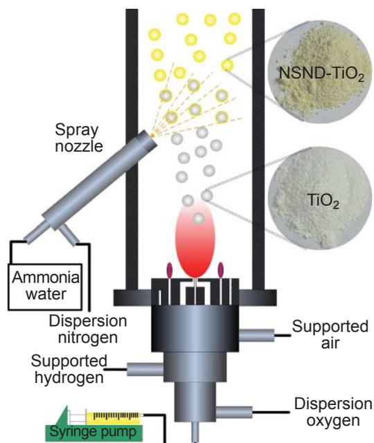
Fig. 7. Schematic setup for N-doped  $\text{TiO}_2$  nanoparticles (Reprinted from (74). Copyright (2014), with permission from Elsevier)
