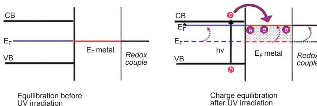
Fig. 2. Equilibration of semiconductor-metal nanocomposites with the redox couple before and after UV irradiation (Reprinted with permission from (25). Copyright (2004) American Chemical Society)
