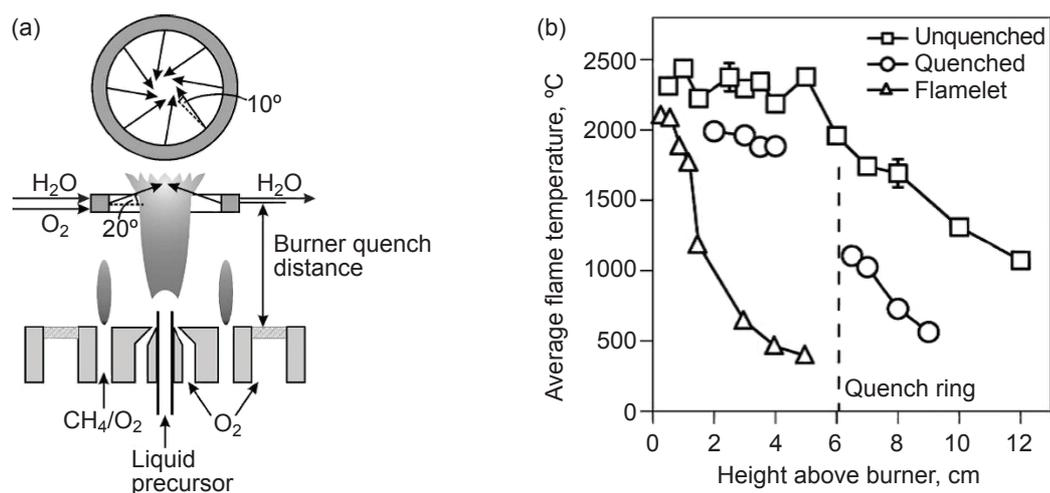
Fig. 5. (a) Burner equipped with a quench cooling device; (b) temperature profiles of the flame spray at standard condition (i.e. unquenched), under quenched condition with a quench ring located at 6 cm above the burner and without precursor feed (49) (Reproduced with permission from Cambridge University Press)
