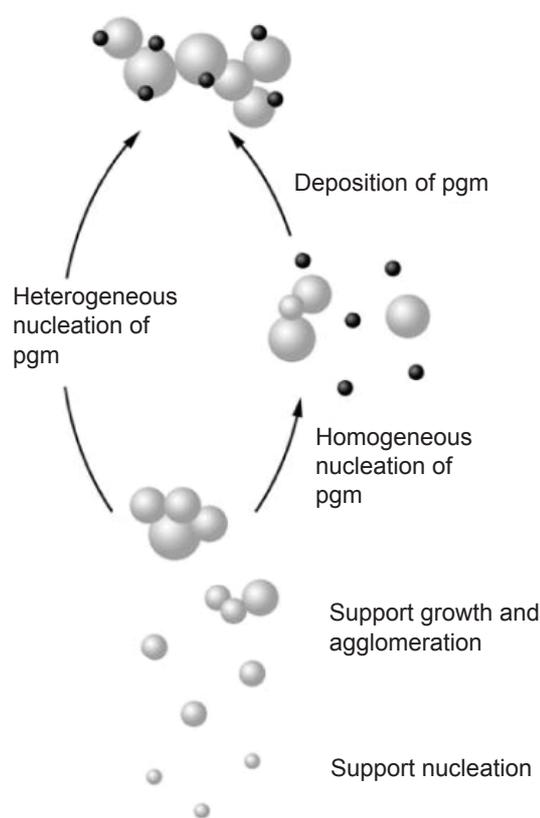
Fig. 3. Mechanism of deposition of p gm on metal oxide substrate in the flame (30)
