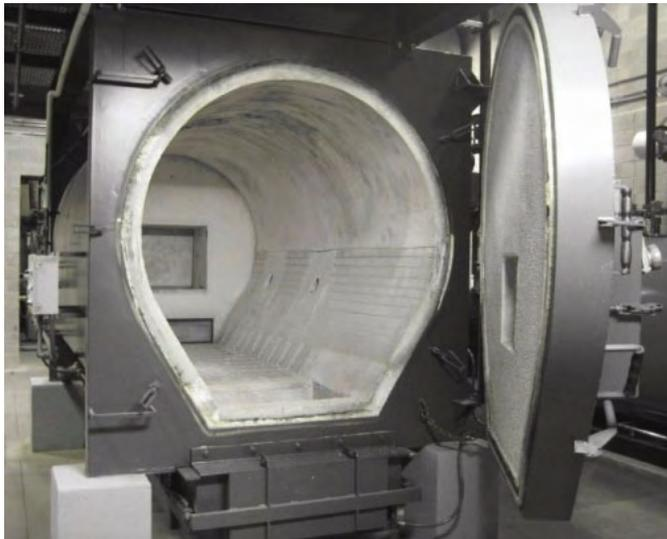
Fig. 3 “The Ox”, a thermal oxidation system for the incineration of precious metal-containing combustibles (Courtesy of Mitch Coughlin, Colt Refining, U.S.A.)
