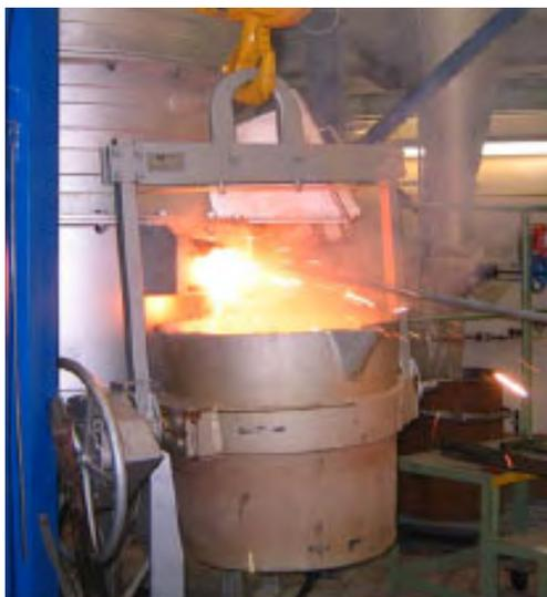
*Fig. 1 Direct-current plasma arc reactor used in the PlasmaEnvi<sup>®</sup> process for the recovery of precious metals from spent refinery catalysts (Courtesy of Martin Bousa, SAFINA, Czech Republic)*
