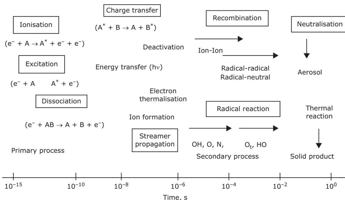
Fig. 2. Timescale for different reactions in plasma. Reprinted from (2), Copyright (2002), with permission from Elsevier
