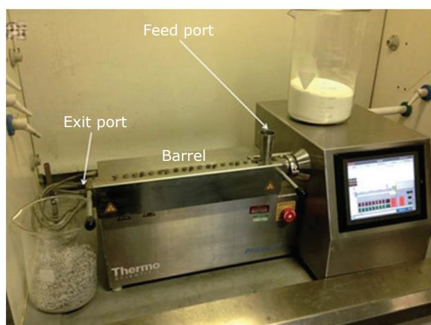
Fig. 1. Twin screw extruder with key parts highlighted. The two screws which convey and knead the reactants are housed in the barrel (4).
