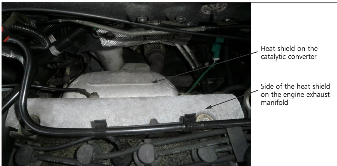
*Fig. 3. A photograph illustrating where a three-way catalyst (TWC) can be mounted directly on the engine exhaust manifold in a modern car. In this position the catalyst can be rapidly heated when the engine is started with a suitable start-up strategy. Since it runs hotter than if it were located further from the engine, less pgm is required than otherwise would be the case. However the high temperatures mean that catalyst thermal durability is essential*
