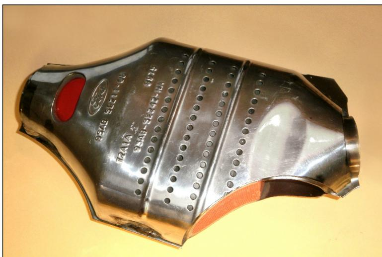
Fig. 2. Photograph of a cut-away three-way catalyst (TWC) converter of a type much used by Ford in Europe in the early 1990s. For a long time two separate TWCs were contained in one can, perhaps reflecting the time when two separated catalysts were used with different functions
