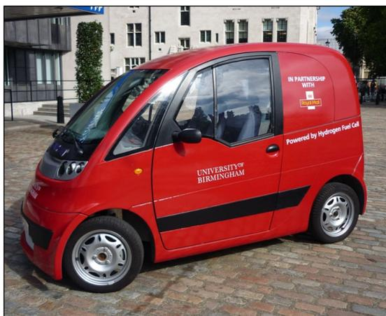
Fig. 4. One of a fleet of five PEM fuel cell/battery hybrid delivery vehicles in daily use on the campus of the University of Birmingham, UK
