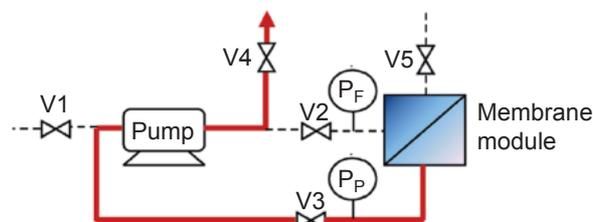
Fig. 4. Pressure-vacuum swing permeation process as reported in (6). Red line shows the path for permeate evacuation (Reprinted with permission from (6). Copyright 2014 Elsevier)
