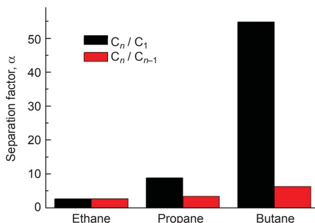
Fig. 2. Highest  $C_4/C_1$  membrane separation, plotted from data reported in (4)
