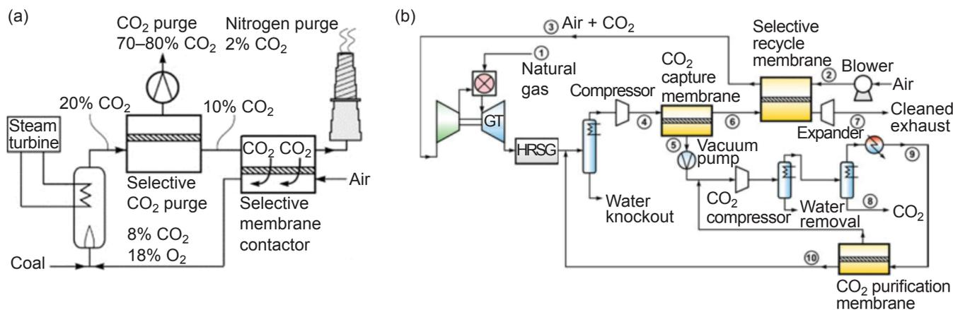
Fig. 1. Block flow diagram of MTR's proposed post-combustion carbon capture in: (a) an integrated gasification combined cycle power plant (Reprinted with permission from (2). Copyright 2014 Elsevier); and (b) a natural gas combined cycle power plant (Reprinted with permission from (3). Copyright 2013 American Chemical Society)
