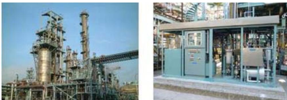
Fig. 3. JX-Nippon Oil and Energy's IPA production plant and the bench-scale zeolite membrane located beside the plant (Image courtesy of Masahiko Matsukata, Waseda University, Japan (5))
