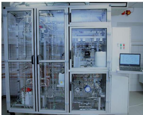
Fig. 3. Small-scale pilot plant for the production of DME from biogas and hydrogen
