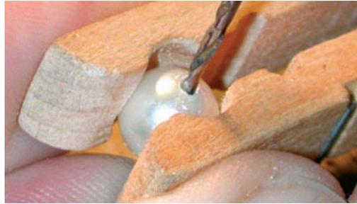
*Using a clothes peg as a multipurpose vice to assemble a pearl to its post (Courtesy of MJSA Press)*
