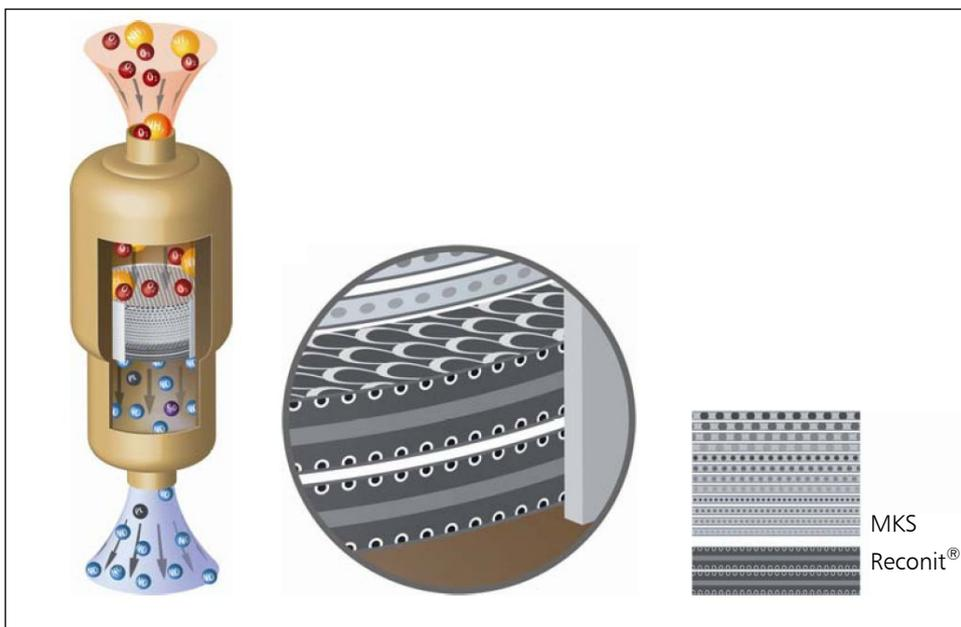
Fig. 2. High pressure reactor for the catalytic oxidation of ammonia with Reconit<sup>®</sup> layers below the MKS Modulares Katalysator System<sup>™</sup> (Courtesy of Umicore, Germany)
