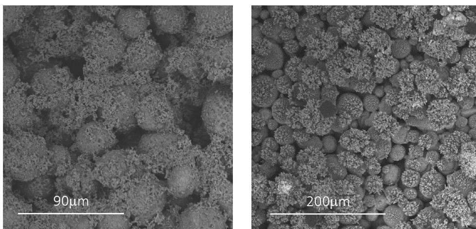
Fig. 3. Different palladium salts give varying coverage of reduced palladium on a stainless steel substrate (Courtesy of Bill Gleason, Montana Tech)
