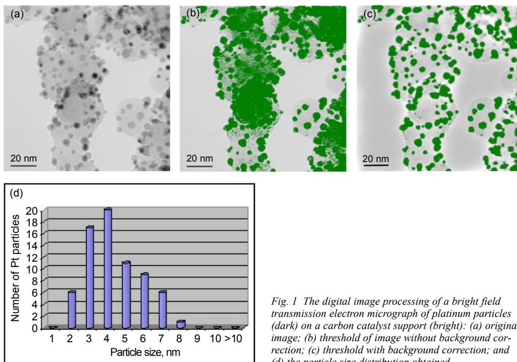
Fig. 1 The digital image processing of a bright field transmission electron micrograph of platinum particles (dark) on a carbon catalyst support (bright): (a) original image; (b) threshold of image without background correction; (c) threshold with background correction; and (d) the particle size distribution obtained
