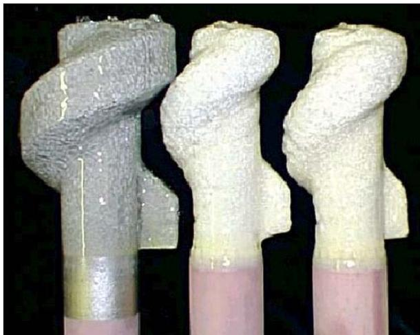
stirrer cores and similar applications in the glass industry have included platinum alloy coated, high strength oxide dispersion strengthened (ODS) superalloys, but without significant success. However, the recent development of ‘diffusion choke’ technology has overturned these failures and enabled the use of these superalloys. This paper looks at the background to the ‘diffusion choke’ development and the improvements that are now possible.
