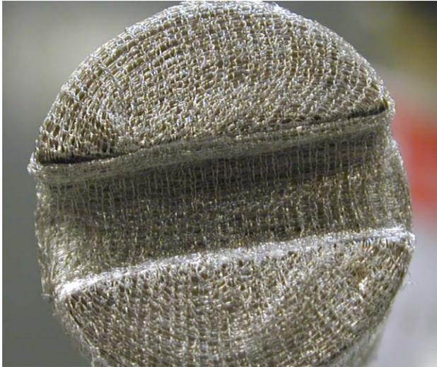
Fig. 6 The typical structure of a knitted 'diffusion choke' gauze or mesh made from 10%Rh-Pt alloy. Here it is wrapped around the core of a stirrer
