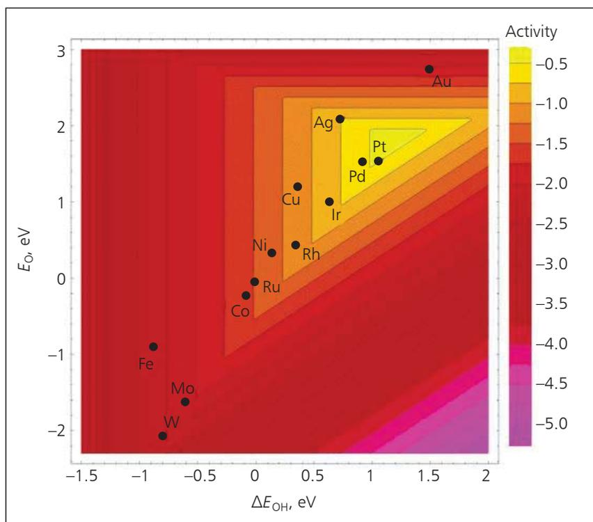
Fig. 1. Trends in oxygen reduction activity plotted as a function of both the O and OH binding energy (1)
