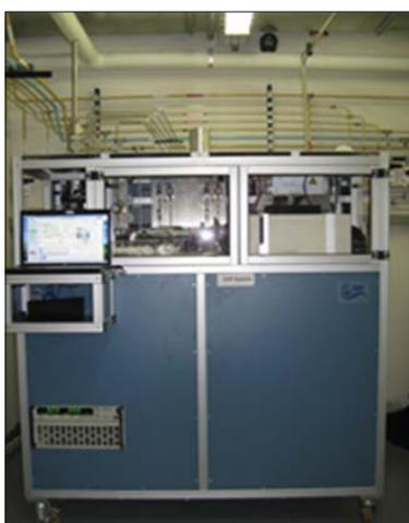
Fig. 6. 2 kW CHP system installed at HySA Systems laboratories
