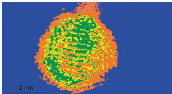
'Core-shell' catalyst where a core of one metal or alloy is encased with a layer of different atoms
