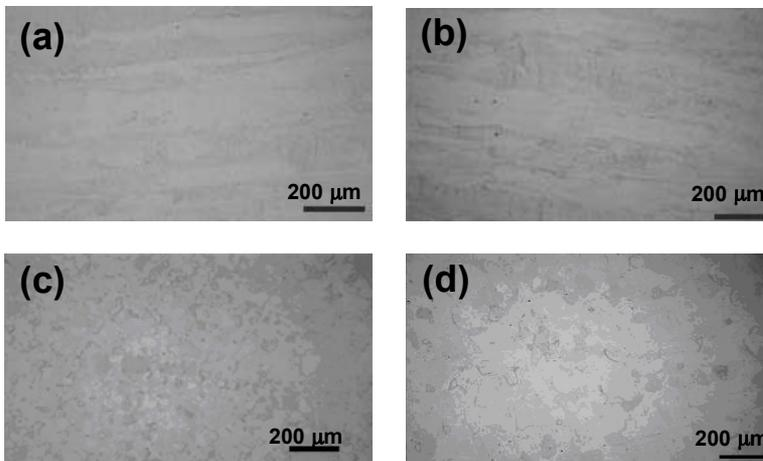
Fig. 4 Micrograph of Pt-5% Cu: (a) 90% cold worked, then heat treated for 3 hours at: (b) 300°C; (c) 700°C; (d) 1000°C
