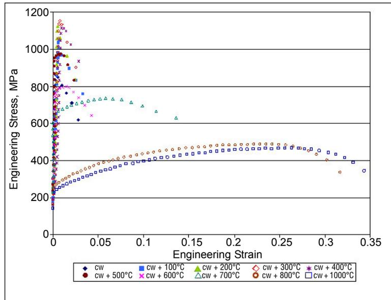
Fig. 2 Extract from Figure 1: Stress-strain curves for Pt-5% Cu in the 90% cold worked condition and after heat treatment at 300°C (highest increase in strength) and 1000°C (cw = cold worked)
