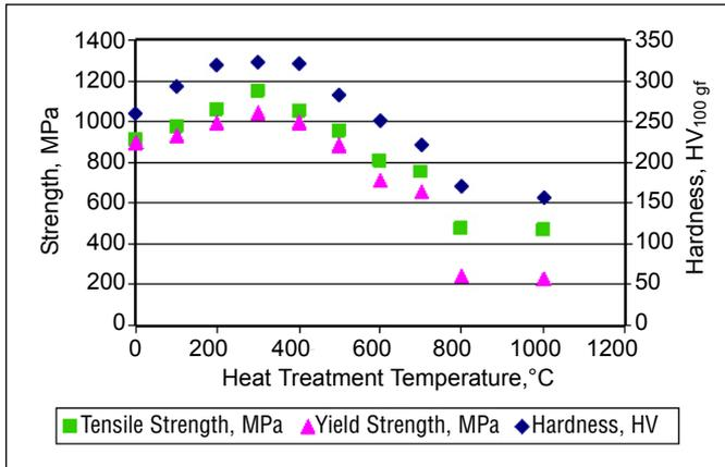
Fig. 3 Mechanical properties of Pt-5% Cu vs. heat treatment temperature after heat treatment for 3 hours
