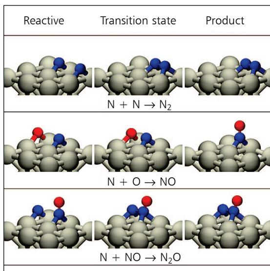
Fig. 2. Representation of the initial, transition and final states for  $N_2$ , NO and  $N_2O$  formation during the oxidation of ammonia on platinum(100), used in building a kinetic model of NO oxidation (Image reproduced with permission from (3). Copyright 2008 American Chemical Society)
