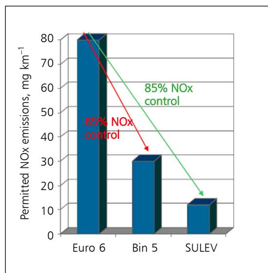
Fig. 1. The US Tier 2 Bin 5 emission standard requires 60% more NO<sub>x</sub> control than Euro 6, and the super ultra low emission vehicle (SULEV) emission category requires 85% more (Courtesy of Tim Johnson, Corning Environmental Technologies, USA)
