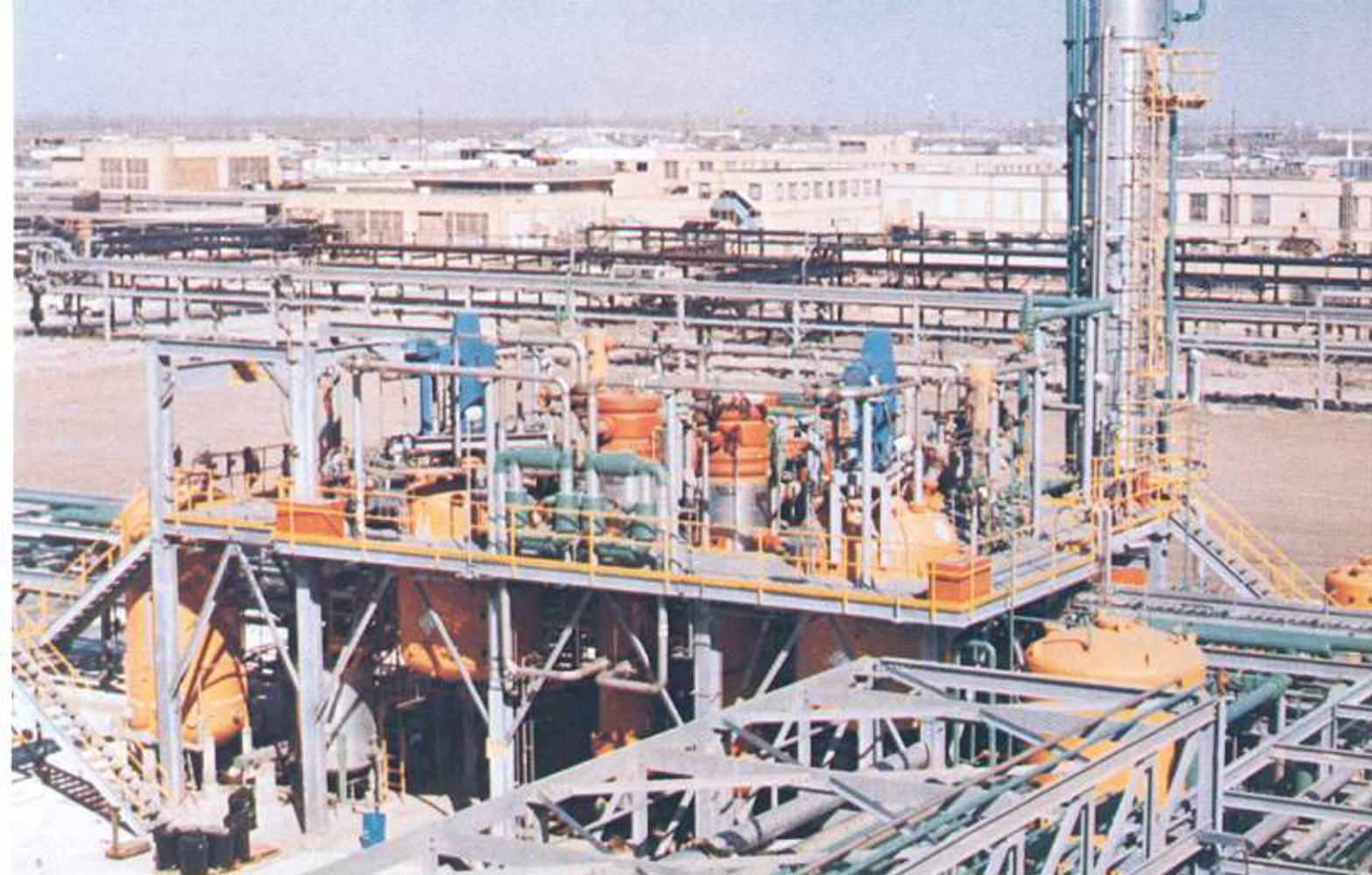
Processing unit of Union Carbide uses new oxo technology to make propionaldehyde from ethylene at Texas City Fig. 6
