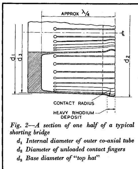
Fig. 2—A section of one half of a typical shorting bridge
