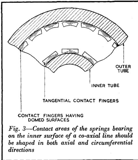
rhodium plated surfaces are in rubbing contact it is always desirable for one of these contacts, in this case the finger contacts, to be dome shaped, but the radius of doming must be large. A small dome will lead to rapid wear owing to scoring of the surfaces by the cutting edge formed as the contact zone wears. Typical minimum radii are usually of the order of 0.125 inch (3 to 4 mm).
