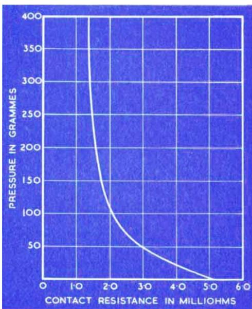
Fig. 1—Effect of increasing pressure on the contact resistance of electrodeposited rhodium
