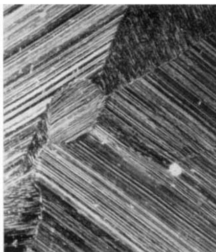
Fig. 2—Striations following crystallographic directions
