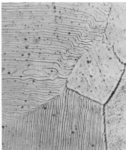
Fig. 4—Striation pattern unchanged by migration of grain boundary  $\times 780$
