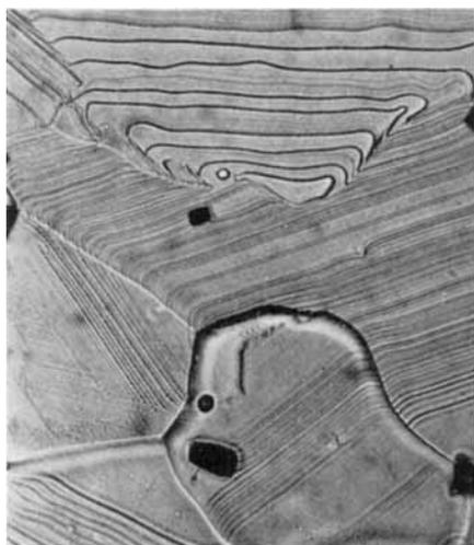
Fig. 3—Curved striations, possibly due to imperfections in the crystals  $\times 780$
