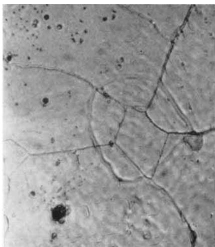
Fig. 1—Traces of grooves at former grain boundaries on a sample which has undergone grain growth
