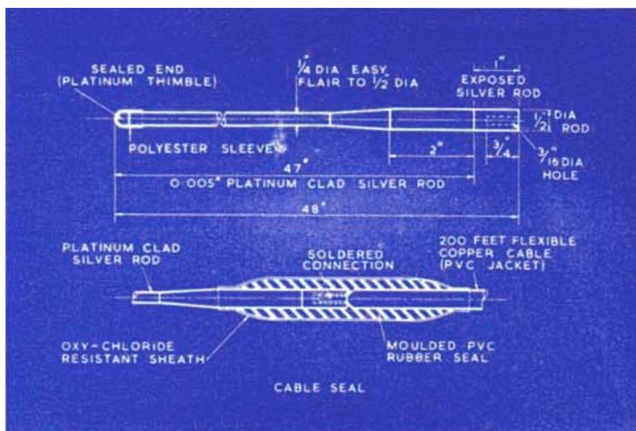
Details of the platinum-clad trailing anode and cable seal
