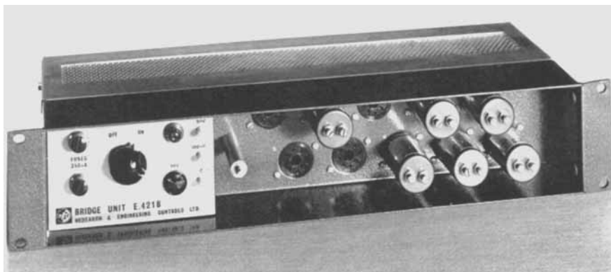
Fig. 8 A versatile 10-channel bridge chassis to which resistance thermometers can be connected. The plug-in double bridge modules convert the resistance change of the sensor to a d.c. output signal suitable for most types of data-loggers and computers
