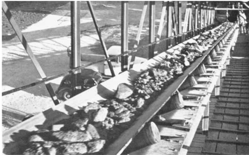
Ore is carried by conveyor belt to the sorting station in the reduction plant
