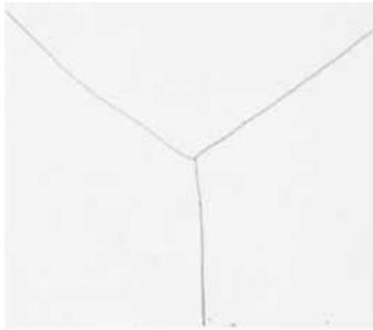
Fig. 2 3 per cent gold-12 per cent rhodium-platinum quenched after annealing for 48 hours at 900°C ( $\times 500$ )
