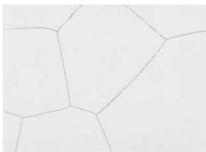
Fig. 5 5 per cent gold-10 per cent rhodium-platinum quenched after annealing for 24 hours at 1200°C ( $\times 500$ )
