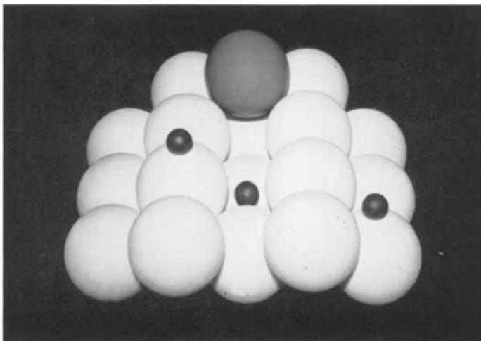
Fig. 5 Model of the (110) face, showing one metal atom in the next layer, and three locations for hydrogen atoms
