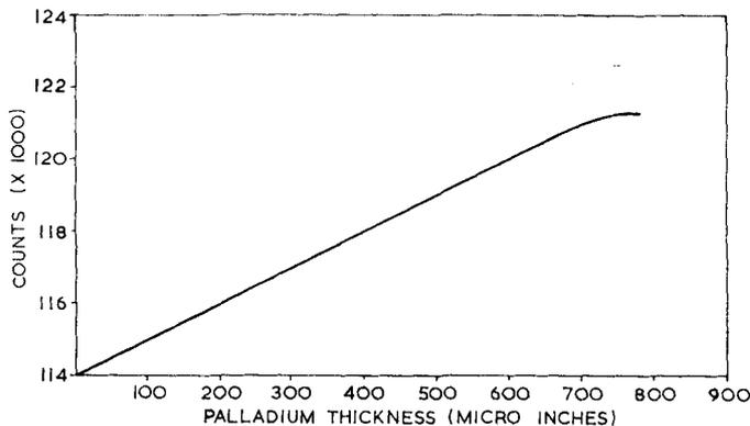
Fig. 3 A calibration graph for palladium plating on copper (Aperture 0.06 inch diameter; counting time 60 seconds)
