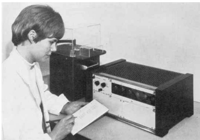
*Fig. 1 For the accurate and non-destructive measurement of plating thicknesses of the platinum group metals the Beta 750 provides a simple and compact instrument, using the principle of "back-scatter" of beta particles*
