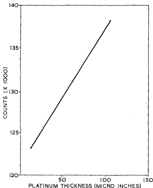
Fig. 2 A typical calibration graph for use with the Beta 750. This shows the thickness of platinum plating on titanium obtained from measurement of standard specimens. (Aperture 0.06 inch  $\times$  0.2 inch; counting time 60 seconds)
