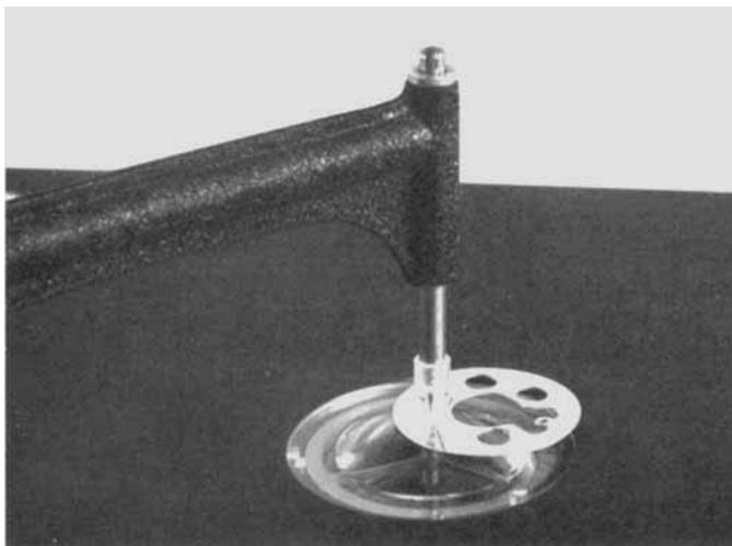
Fig. 4 A close-up view of the measuring head being used to determine the thickness of a rhodium electrodeposit on nickel
