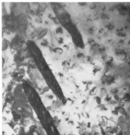
Fig. 1 The structure of a titanium-0.15 per cent palladium alloy showing elongated particles of a  $Ti_2Pd$  phase ( $\times 55,000$ )
