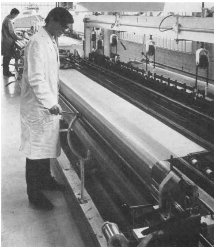
*Fig. 7 One of the looms in the Johnson Matthey gauze shop, showing a rhodium-platinum gauze 140 inches (3.56 metres) wide being woven from 0.003 inch diameter wire*
