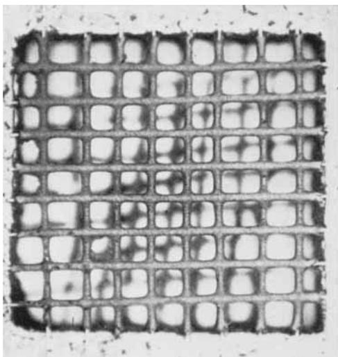
Fig. 2 An experimental  $8 \times 8$  memory array made by depositing ferrite on to platinum wires
