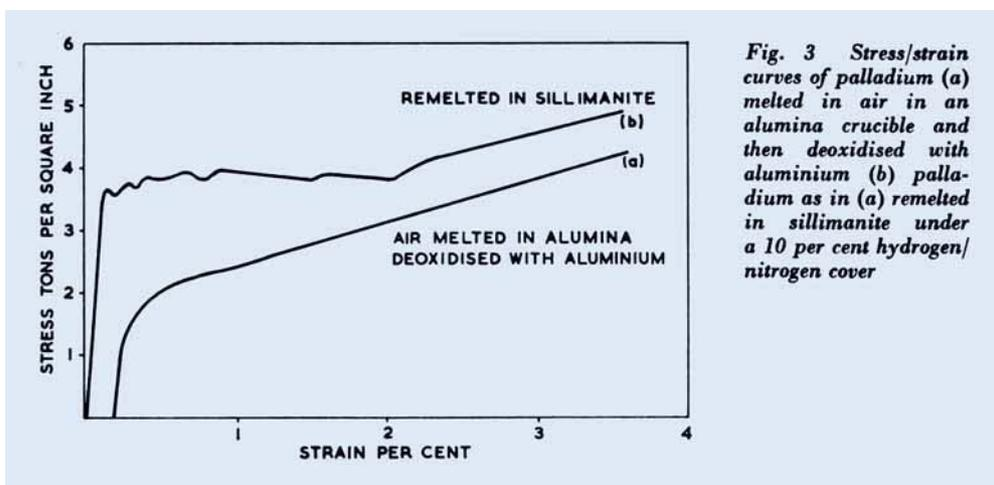
Fig. 3 Stress/strain curves of palladium (a) melted in air in an alumina crucible and then deoxidised with aluminium (b) palladium as in (a) remelted in sillimanite under a 10 per cent hydrogen/nitrogen cover
