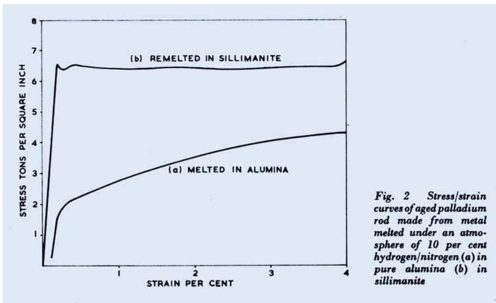
*Fig. 2 Stress/strain curves of aged palladium rod made from metal melted under an atmosphere of 10 per cent hydrogen/nitrogen (a) in pure alumina (b) in sillimanite*
