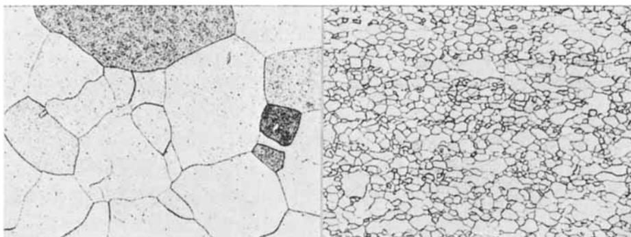
*Fig. 5 Microstructure of fully annealed palladium reduced 20 per cent in area by cold swaging and then aged at 640°C ( $\times 100$ )*
