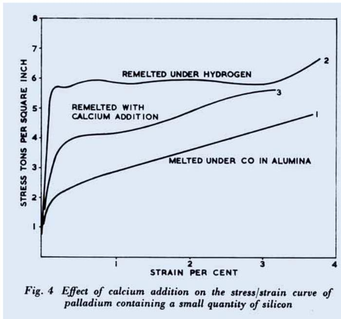
Fig. 4 Effect of calcium addition on the stress/strain curve of palladium containing a small quantity of silicon
