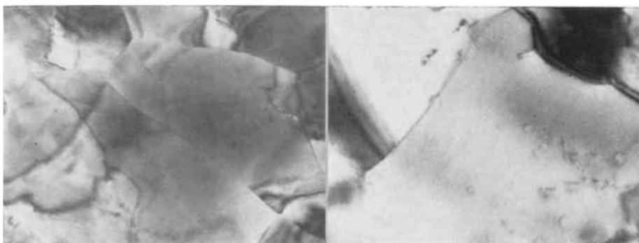
*Fig. 7 Cellular structure of aged section of palladium exhibiting a strong yield point. Silicon content 0.002 per cent ( $\times 100,000$ )*
