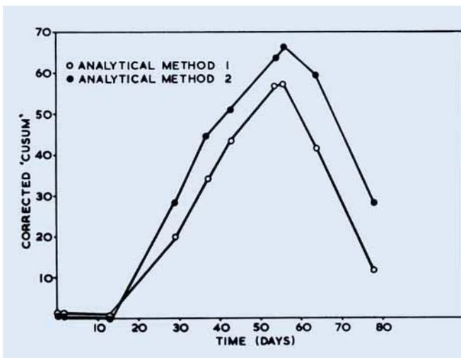
Fig. 2 A cusum plot for one of the ammonia converters, based on a datum of 94 per cent. This shows that to maintain a conversion efficiency equal to the chosen datum it is necessary to pickle the rhodium-platinum gauzes after approximately eighty days
