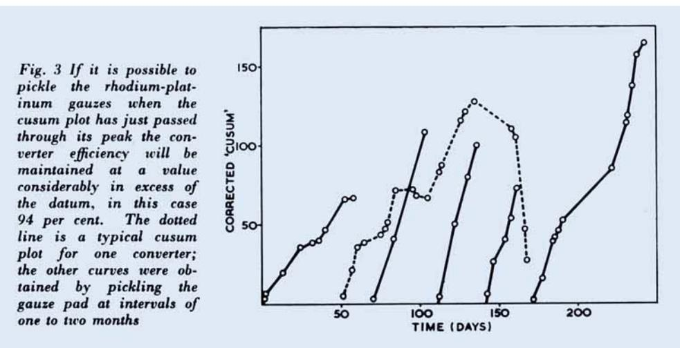
Fig. 3 If it is possible to pickle the rhodium-platinum gauzes when the cusum plot has just passed through its peak the converter efficiency will be maintained at a value considerably in excess of the datum, in this case 94 per cent. The dotted line is a typical cusum plot for one converter; the other curves were obtained by pickling the gauze pad at intervals of one to two months
