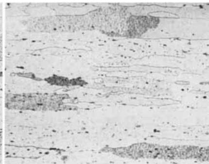
*Fig. 8 Microstructure of sheet, recrystallised at 1400°C after the ingot from which it had been produced was directly cold rolled. The total reduction imposed by cold working was 90 per cent ( $\times 150$ )*
