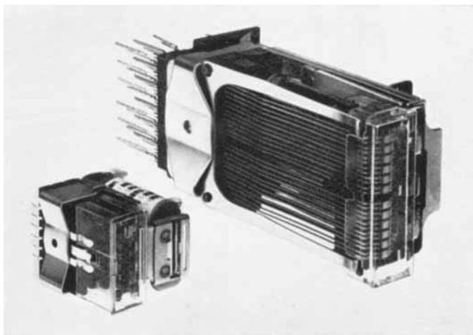
*The contact arrangement in the miniature wire spring relay*
