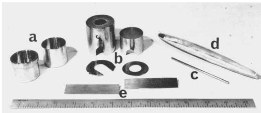
Fig. 3. Platinum metal ware used in the growth of oxide single crystals
