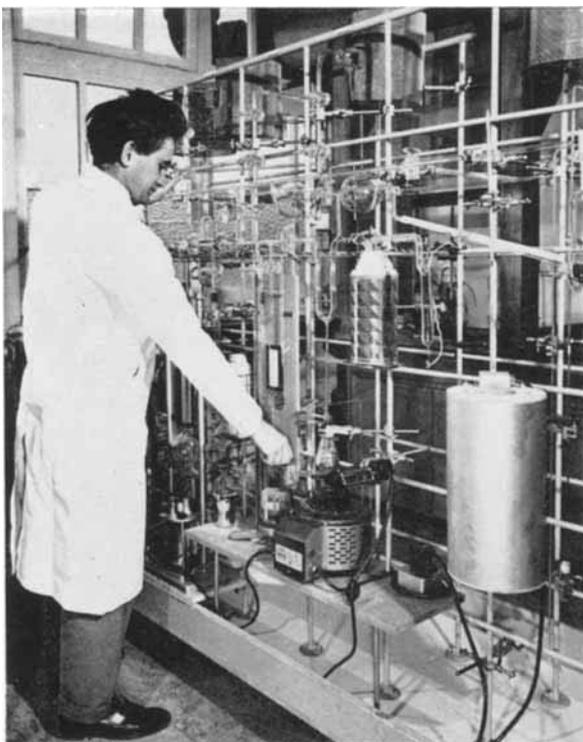
*Research into the mechanism of chemical reactions involving platinum group metal catalysts, and into the variables that need to be controlled, is carried out in apparatus of this type*
