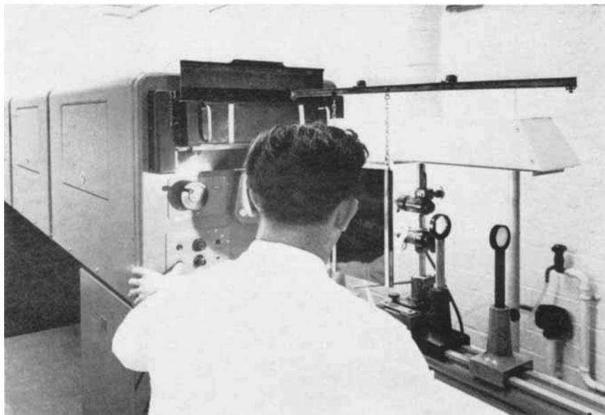
*One of the modern spectrographs, a 3.4 metre Ebert grating instrument, which facilitates the detection and accurate determination of trace impurities in the platinum metals*
