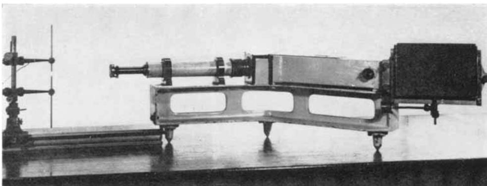
*The Hilger medium spectrograph purchased in 1920, initially for the determination of iron in rhodium. Since that time a wide range of spectrographic instruments has been installed*
