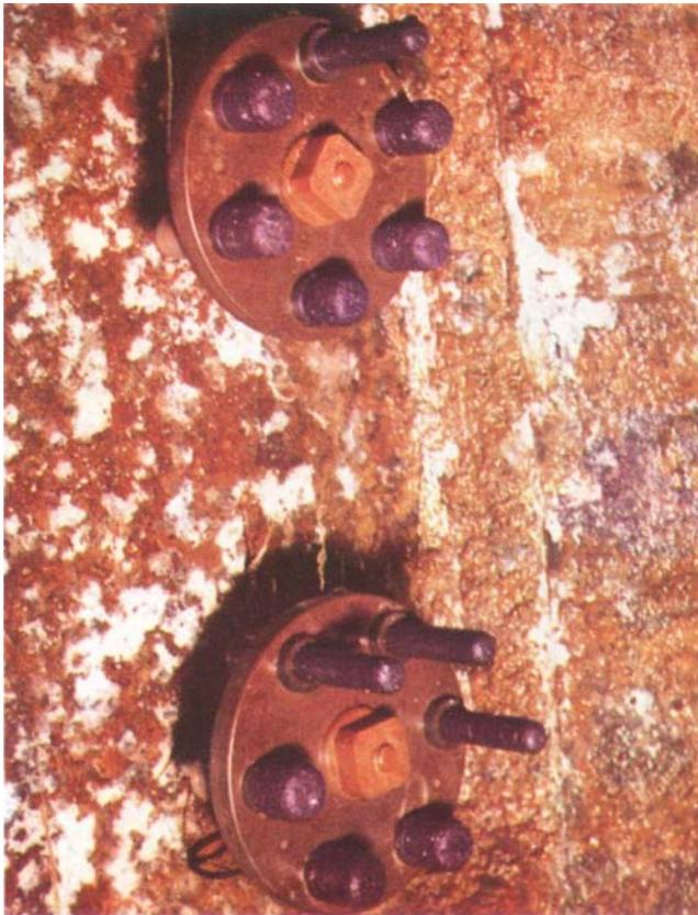
*The type of lead or lead alloy for use in platinum bielectrodes is important, and extensive tests have been carried out with a number of alloys. The anodes shown here were in use for a year, at 50 amps per square foot, in a water box at Marchwood Power Station in order to assess the effect of composition on the growth and spalling of the lead peroxide*
