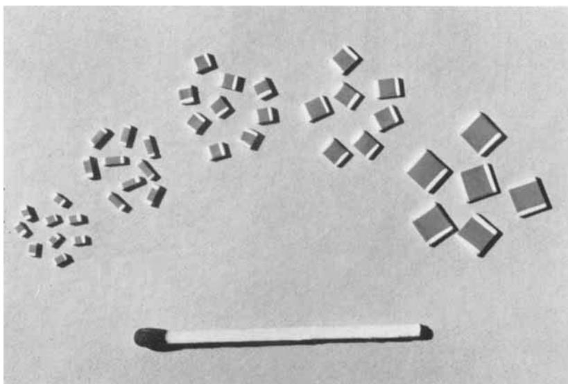
*Some of the K1200 and NPO monolithic ceramic capacitor chips from Matthey Printed Products Limited. The smallest is  $2.4 \times 1.3 \times 1.3$  mm, the largest  $9.9 \times 10.8 \times 1.7$  mm, offering in all a capacitance range of 5.6 to 470,000 pF at a peak rating of 100 volts. The terminal areas are metallised to facilitate soft soldering.*
