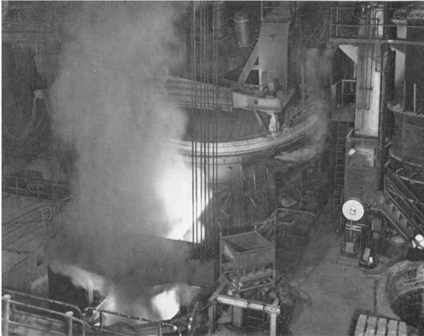
*Fig. 2 After a lengthy evaluation of the expendable cartridge technique in the electric arc furnaces at Steel, Peech & Tozer three sets of equipment have been installed and substantial time savings have been made in routine working*
