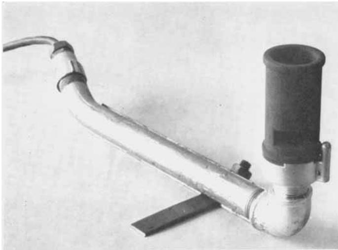
*Fig. 3 In order to make a determination the cartridge is mounted in a metal stand to enable the thermocouple to make contact with the compensating cable linking it to a temperature recorder*
