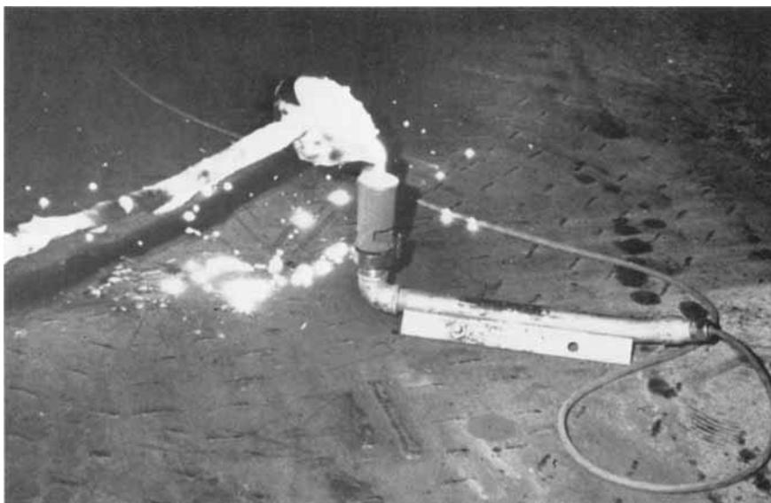
*Fig. 5 In order to take a reading a sample of molten steel is poured into the Tectip cartridge. The thermal arrest point is recorded within twenty seconds, and the carbon content can then be read from a conversion graph fully corrected for the effects of other elements*
