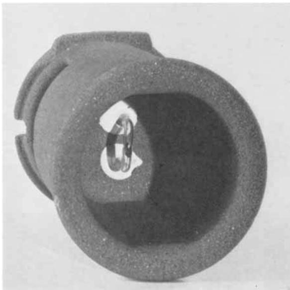
*Fig. 1 The Leeds & Northrup Tectip S cartridge for the rapid determination of carbon in liquid steel. The platinum:rhodium-platinum thermocouple can be seen through the transparent quartz tube fitted into the bottom of the sand mould*
