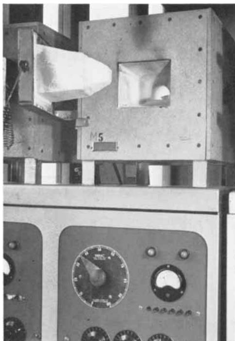
*Fig. 2 A complete muffle furnace with its proportional controller*
