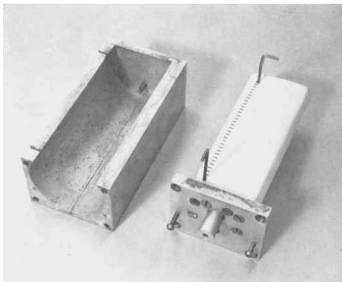
*Fig. 1 The mould and former for a D-shaped element of internal dimensions 12.5 × 5 × 3.5 cm. The paper covering the former is marked ready for winding the 20 per cent rhodium-platinum wire.*
