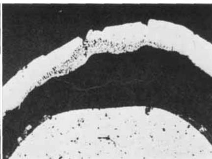
*Fig. 8 A grain boundary failure within the sheath of a specimen which was rapidly losing weight.  $\times 25$*
