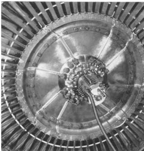
*A typical assembly of eight strain gauges fitted to a turbo-jet engine*
